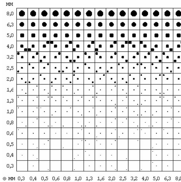
Figure 2: The CDRAD-phantom, presented in a schematic way [11].
