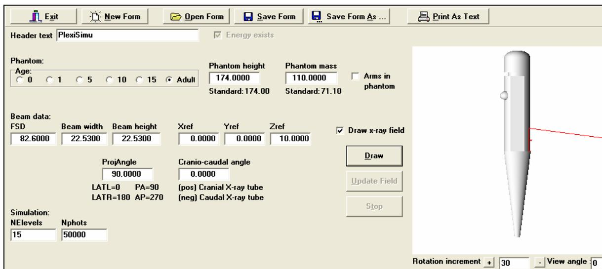
Figure 4: The setup in PCXMC to simulate the effective dose during the phantom study
