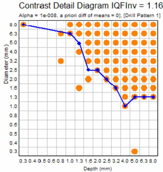
Figure 3: The contrast-detail diagram and curve as shown by the CDRAD Analyser.
