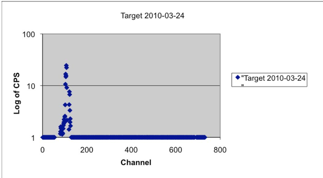
**Plot 9:** Spectrum of the HPGe detector of the target 2010-03-24.
