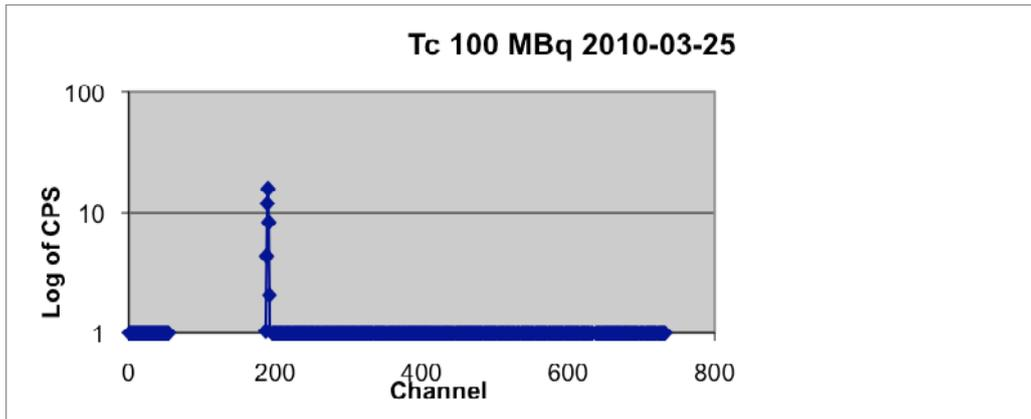
**Plot 12:** Spectrum from the HPGe detector of a scintillation vial with a solution of PBS and 100 MBq  $^{99m}\text{Tc}$ .
