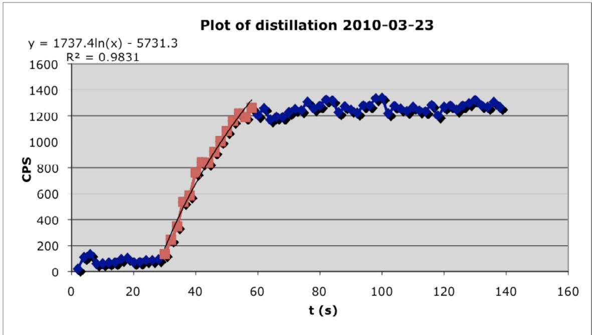
**Plot 2:** Distillation plot for measurement 2010-03-23. A trend line for the rapidly growing first part of the process is included.
