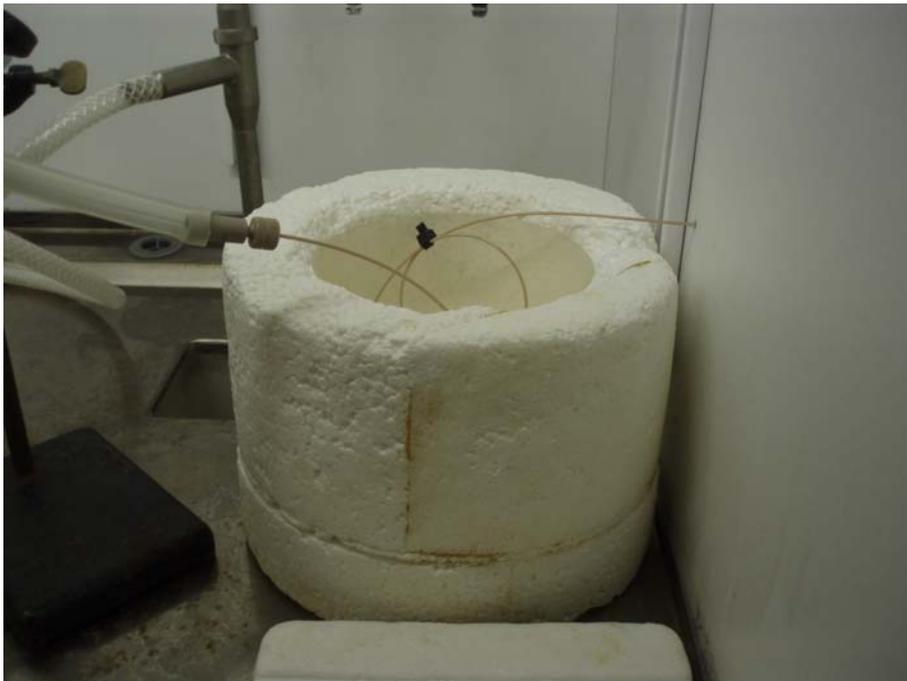
**Figure 6:** *The PEEK tube from the oven (through the hole to the right) leading down into the Styrofoam cylinder.*
