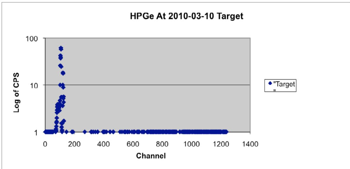
**Plot 6:** Spectrum from the HPGe detector of the  $^{211}\text{At}$  target 2010-03-10.
