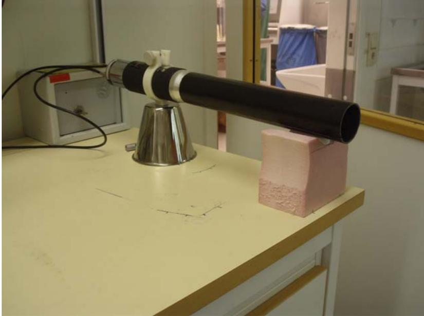
**Figure 3:** *The NaI detector with the lead collimation and Styrofoam support. The detector was positioned on a bench approximately two meters from the measuring point.*
