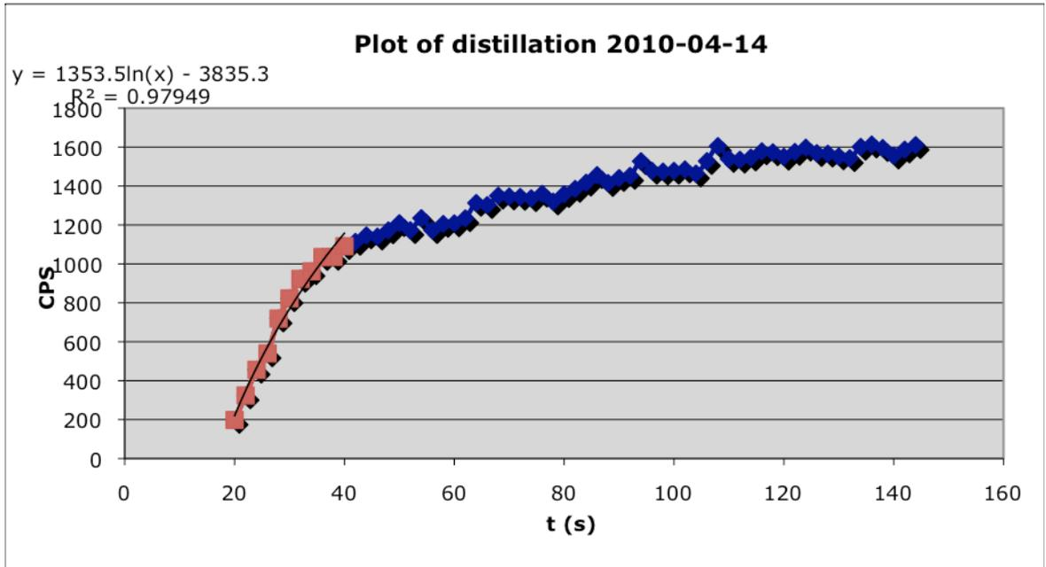
**Plot 4:** Distillation plot for measurement 2010-04-14. A trend line for the rapidly growing first part of the process is included.
