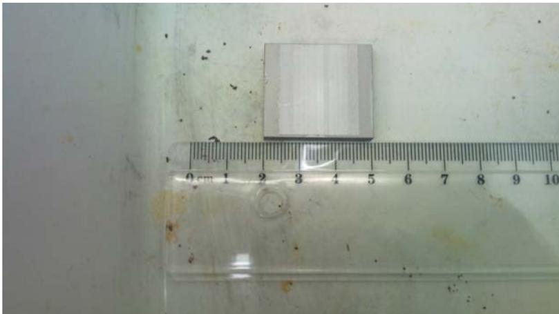
**Figure 2:** *The target as it were after the <sup>211</sup>At was removed.*
