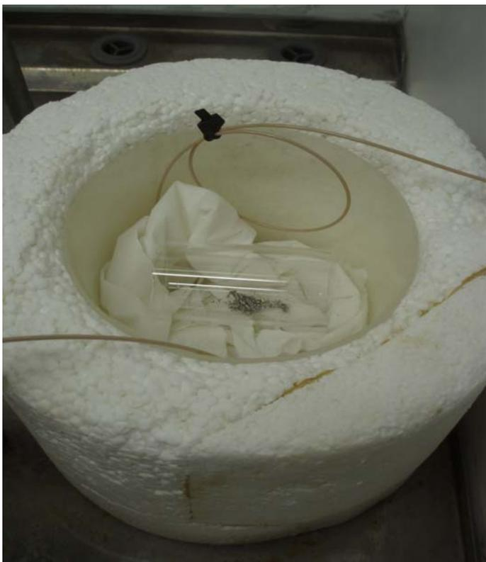
**Figure 5:** *The scrapings in the quartz boat. To be able to balance the boat, it was placed on bunched up paper. An empty PEEK tube (used in the distillation process) is noticeable in behind the boat.*
