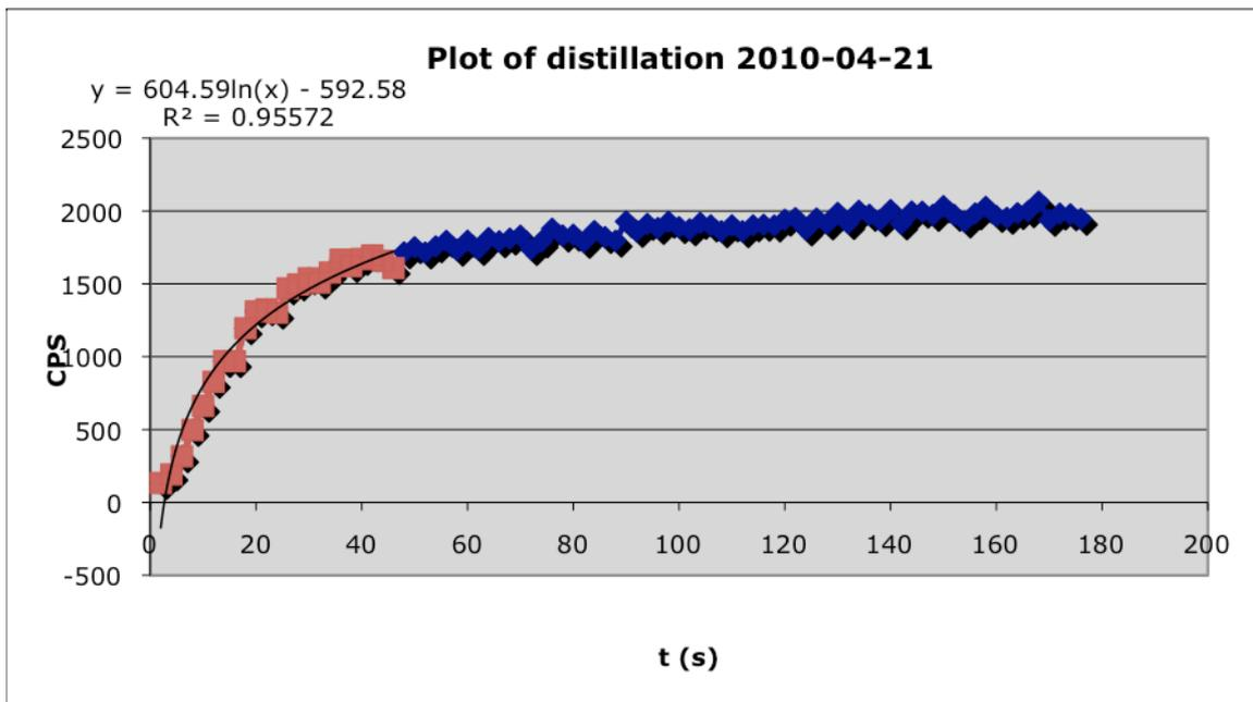
**Plot 5:** Distillation plot for measurement 2010-04-21. A trend line for the rapidly growing first part of the process is included.
