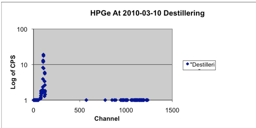
**Plot 8:** Spectrum of the HPGe detector of the distillation process 2010-03-10.
