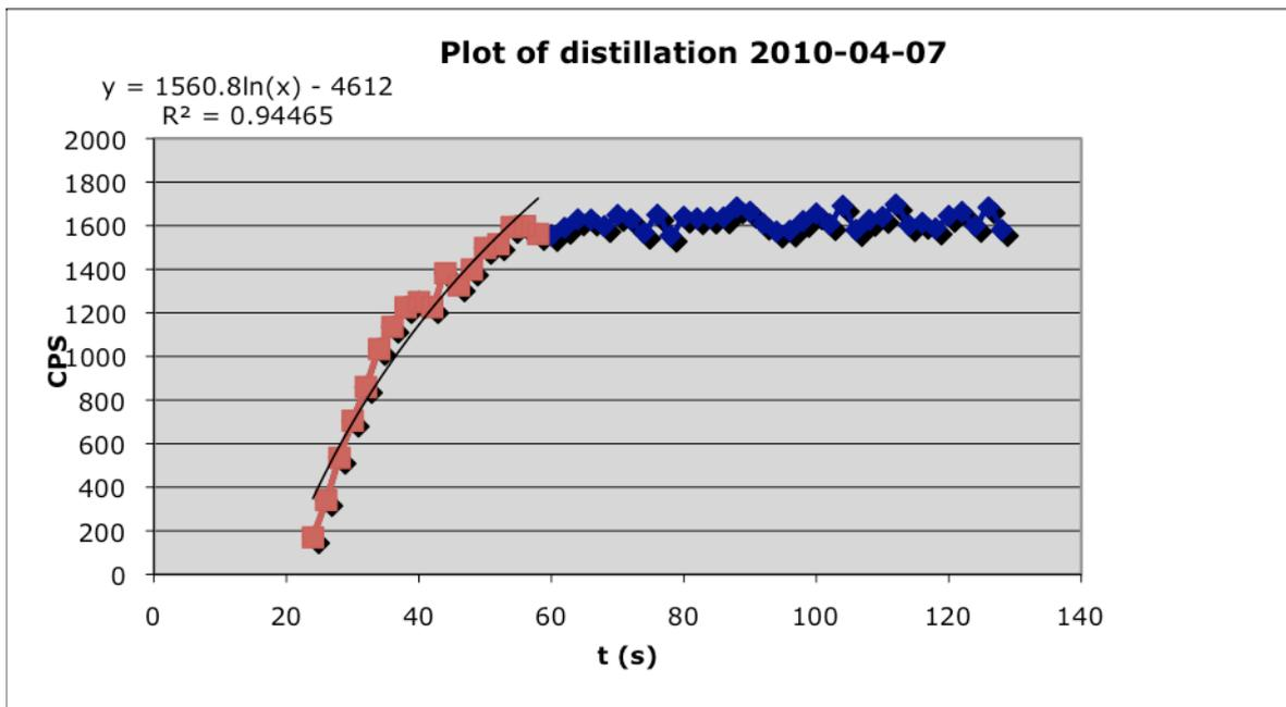
**Plot 3:** Distillation plot for measurement 2010-04-07. A trend line for the rapidly growing first part of the process is included.
