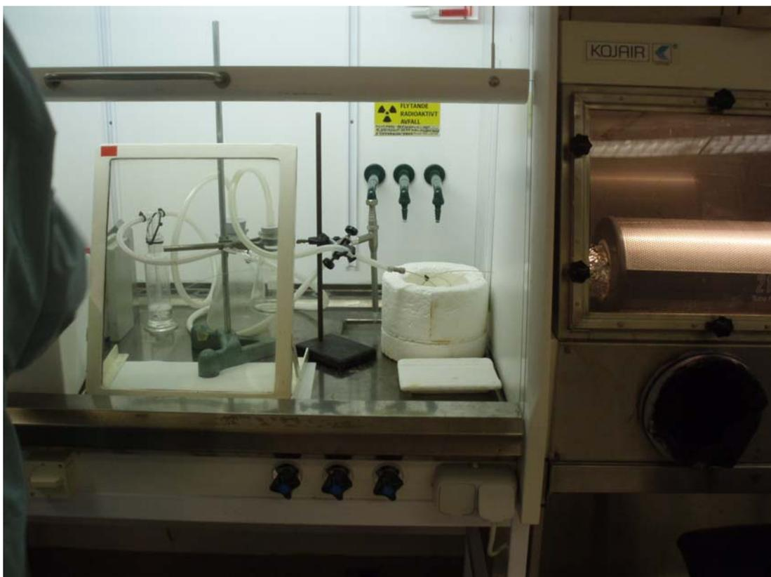
**Figure 8:** *The Styrofoam cylinder filled with dry ice + ethanol and the back flush safety system consisting of empty E-spots and a measuring glass filled with a binding agent.*
