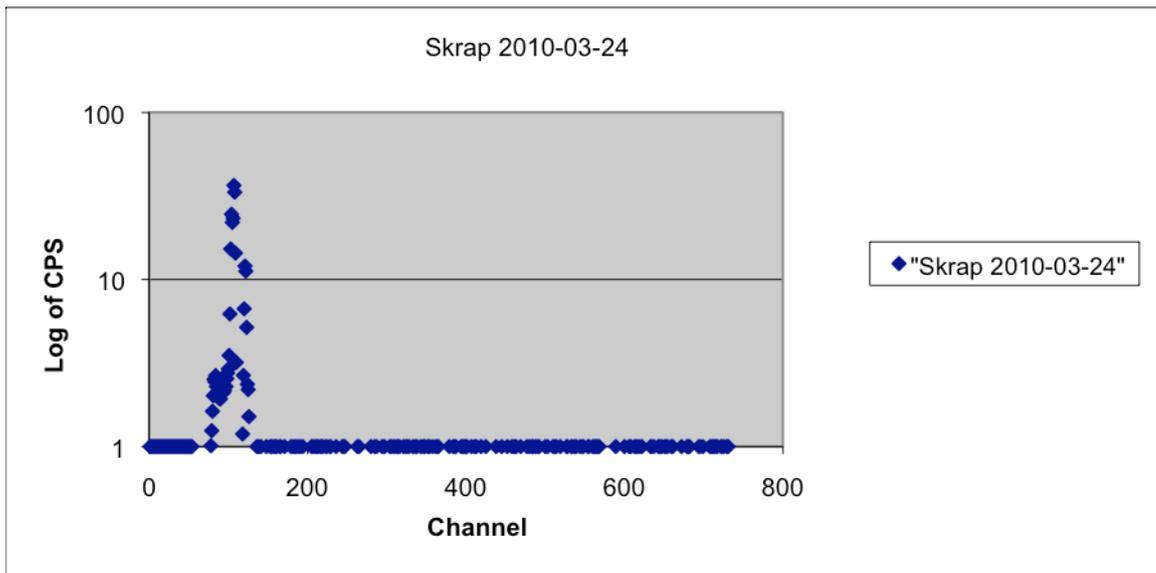
**Plot 10:** Spectrum of the HPGe of the  $^{211}\text{At}$  scrapings 2010-03-24.
