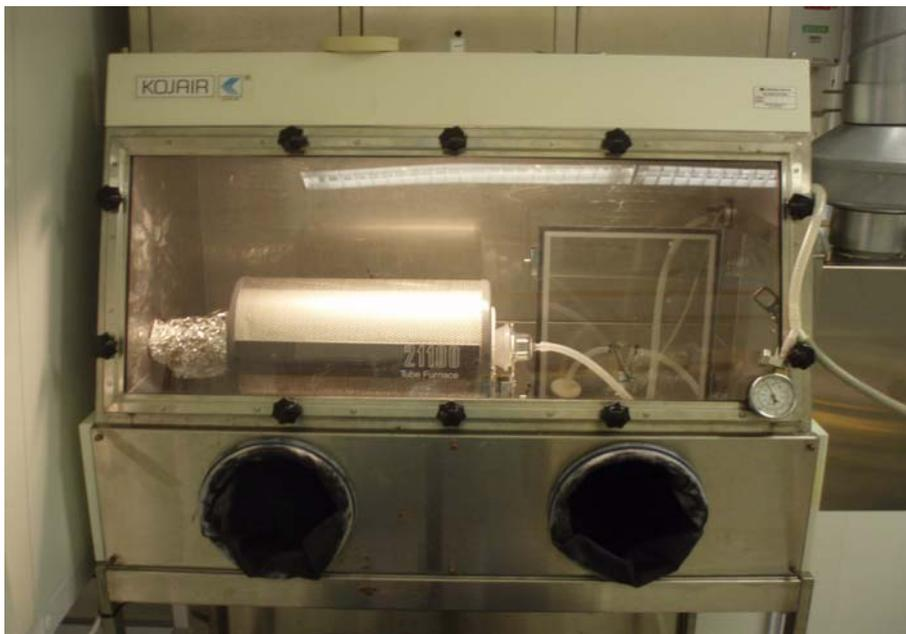
**Figure 7:** *The glass cage with the oven used for distillation of  $^{211}\text{At}$ . The tubing and pressure gate to the right belongs to the nitrogen supply system.*
