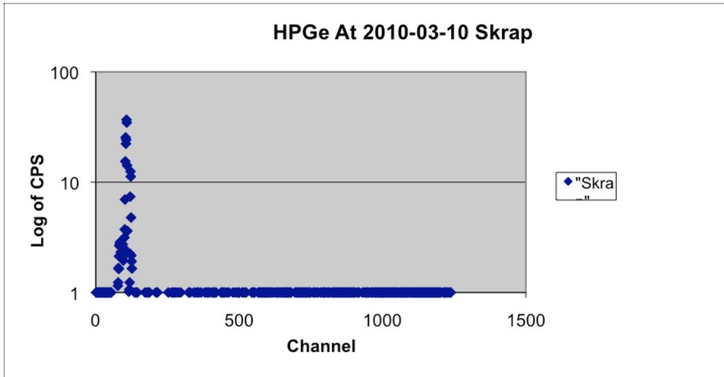
**Plot 7:** Spectrum from the HPGe detector of the  $^{211}\text{At}$  scrapings 2010-03-10.
