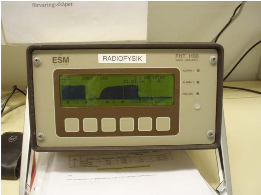
**Figure 4:** *The ESM rate meter.*
