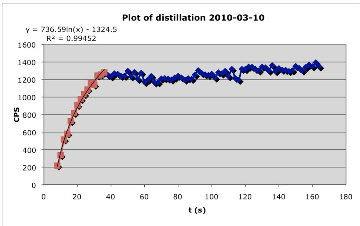
**Plot 1:** Distillation plot for measurement 2010-03-10. A trend line for the rapidly growing first part of the process is included.
