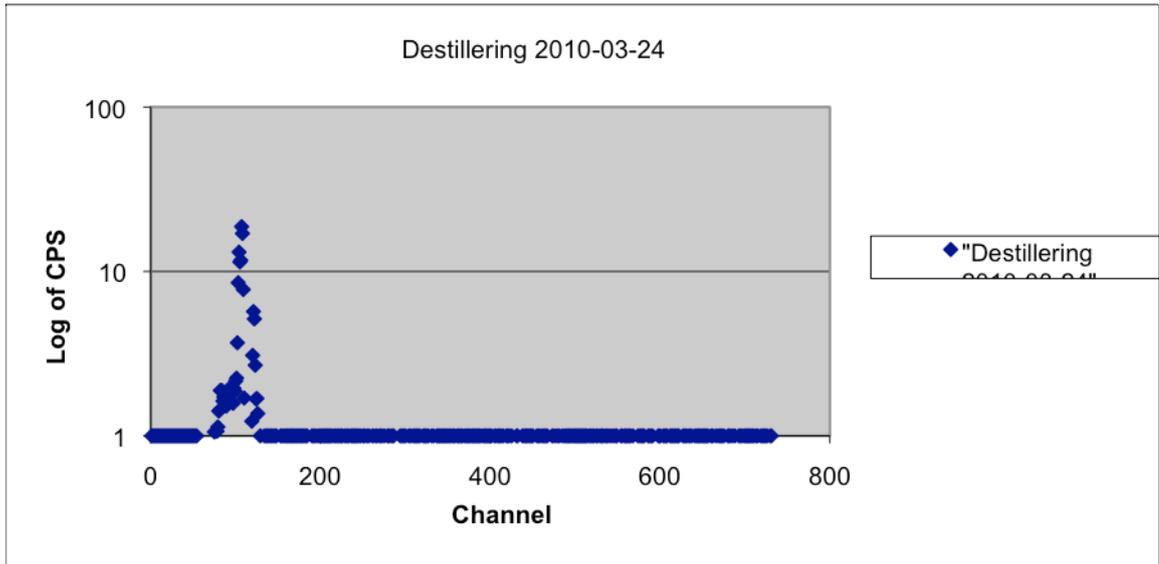
**Plot 11:** *Spectrum of the HPGe of the distillation process 2010-03-24.*
