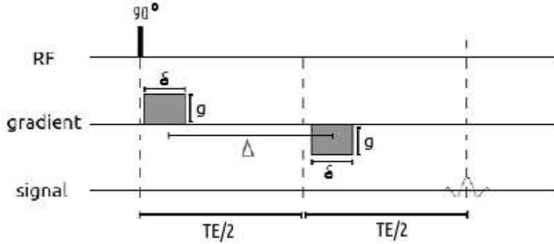
Figure 2.1: A PGSE sequence following an RF pulse. The second gradient pulse causes the particles to rephase and generate a signal maximum after TE.
