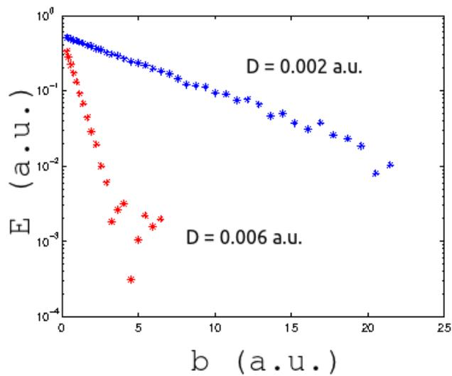
Figure 4.11: Plotted is the echo decay signal  $E$  vs. the parameter  $b$  (see sec. 2.3.2 for definition) for two different cases as indicated of freely diffusing particles.
