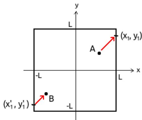
Figure 3.3: In the two dimensional case particles are transposed to the oppsite boundary so that  $x'_1 = -x_1$  and  $y'_1 = -y_1$ .
