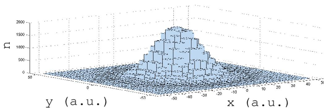
Figure 4.6: Freely diffusing particles in two dimensions. Shown is the distribution after certain diffusion time starting from the origin.
