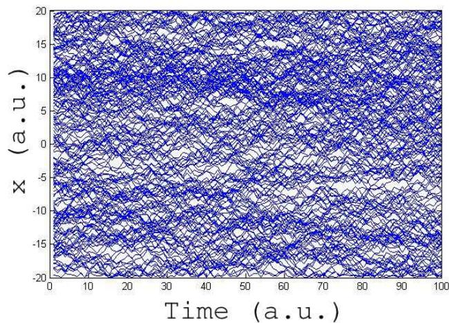
Figure 4.3: The diffusion tracing for particles with free diffusion in one dimension over time. The particle start position is uniformly placed at random in a closed interval.
