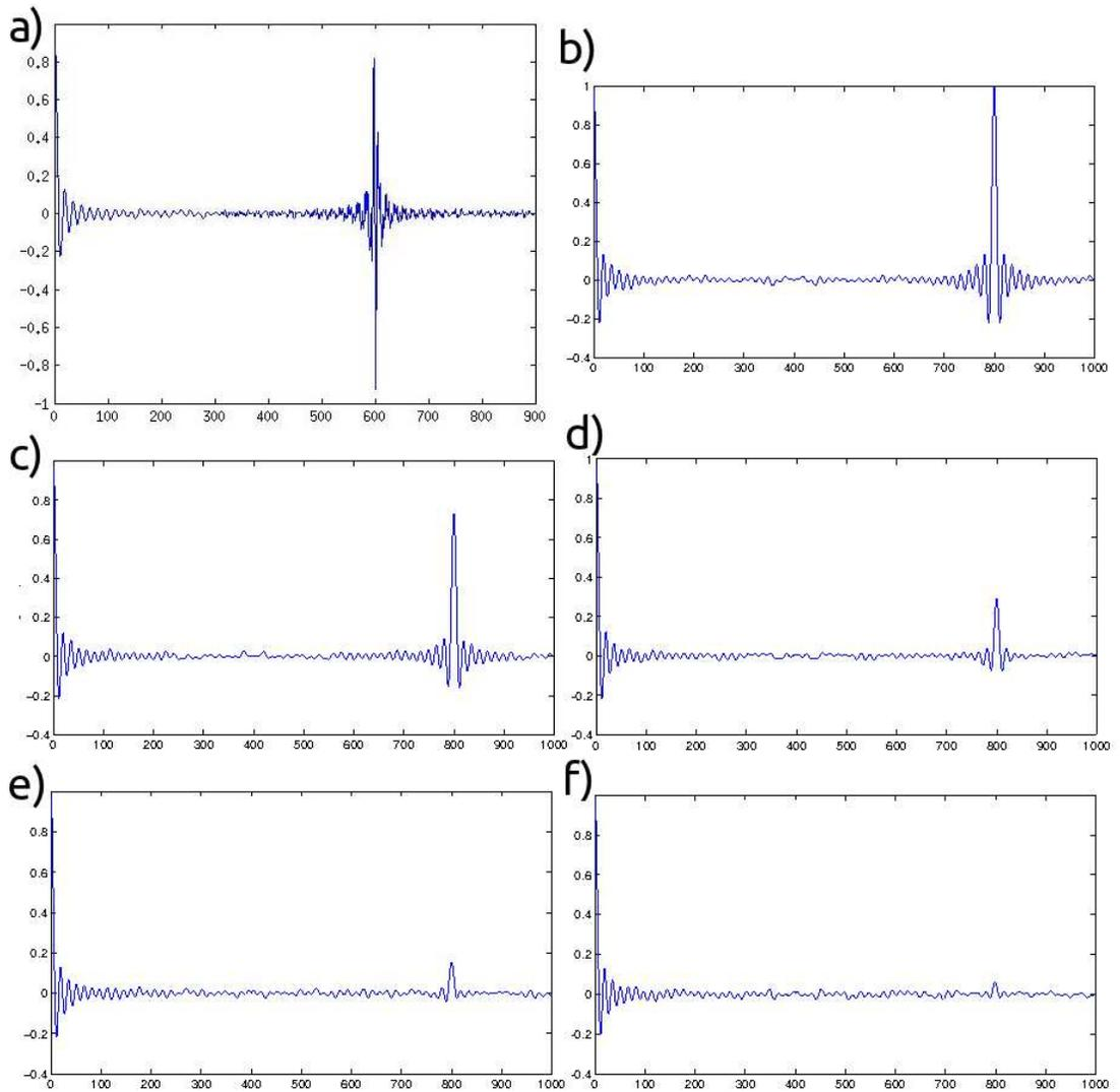
Figure 4.10: Shown is the coil signal for six different cases, a) solid material without diffusion, b)-f) materials with increasing amount of diffusion. Plotted is current (a.u.) vs. time (a.u.). Notice how the echo signal gradually vanishes with increasing diffusion.
