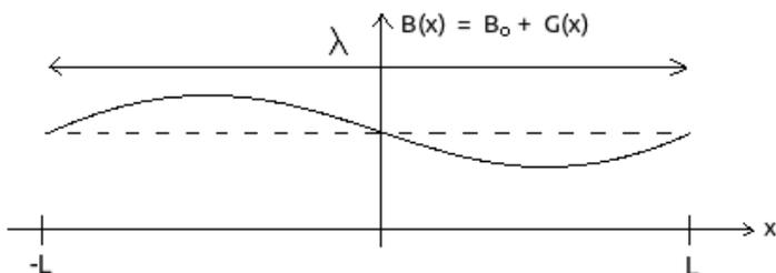
Figure 2.3: Illustrates a sinus shaped gradient field component  $G(x)$  on top of the constant magnetic field  $B_0$  (dashed line). Diffusion boundaries are at  $\pm L$ .
