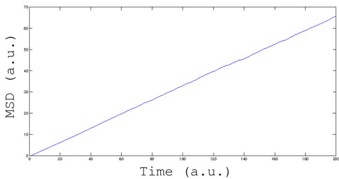
Figure 4.2: MSD for free diffusion particles in one dimension over time.
