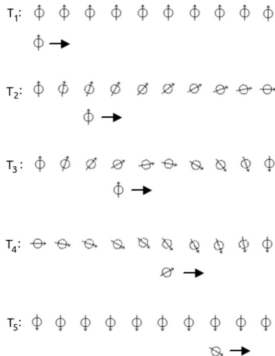
Figure 2.2: Spin orientation as a function of position at five different times. A diffusing particle will however be out of sync.
