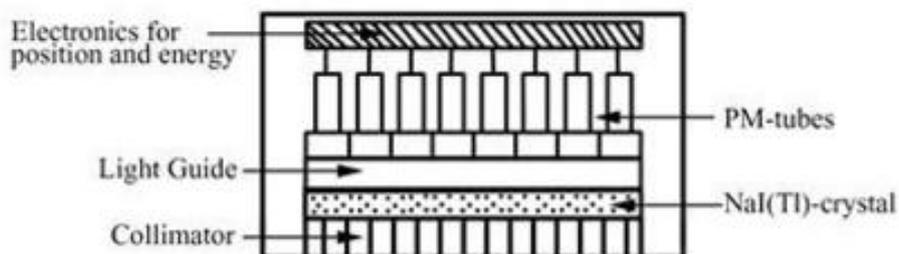
**Figure 1: Schematic picture of the gamma camera.**
