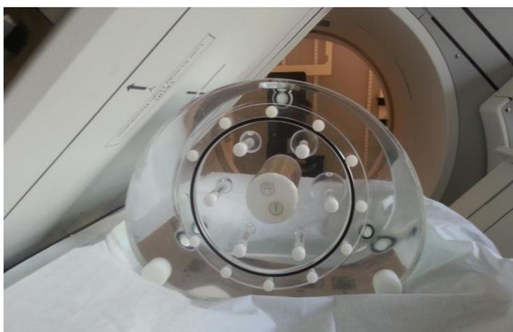
Figure 2: NEMA thorax phantom placed in gamma camera.
